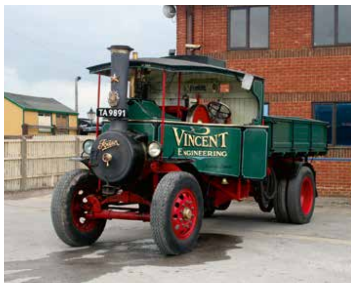
An example of what can be done with very little to start with: Richard 'Turbo' Vincent's lovely Foden steam lorry Freddie was built from the boiler, all other parts being sourced or made by Richard.
