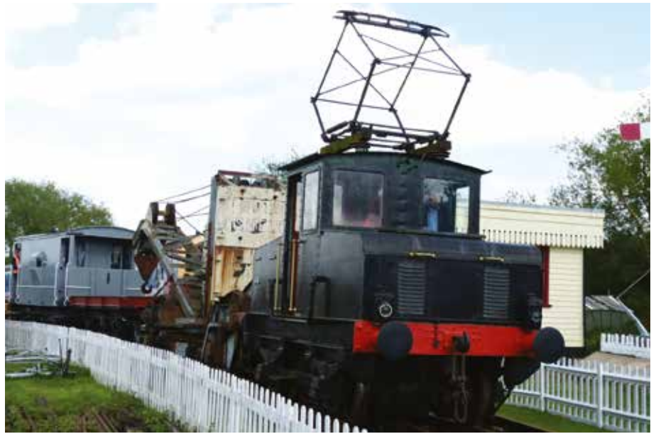
Battery-powered 'Spondon' loco shunting the crane at the Coventry Electric Railway Museum. Brian Hewitt
