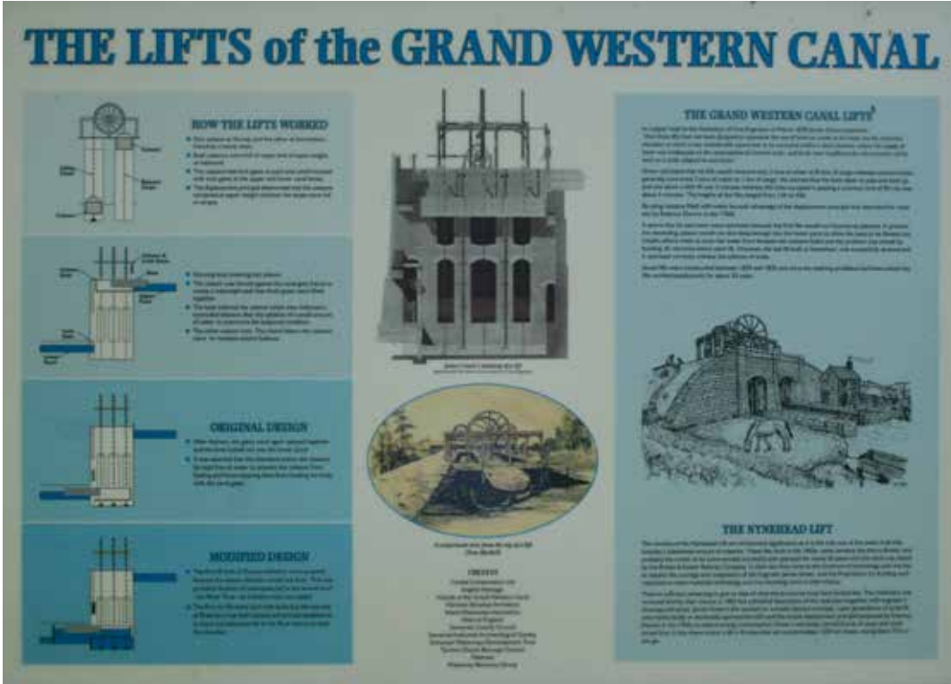
This sign explains the workings of the boat lifts and that at Nynehead in particular.
