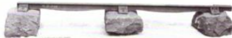
'Fishbelly' rails (so called due to their shape) and stone sleeper blocks like those used on the 1815 waggonway
