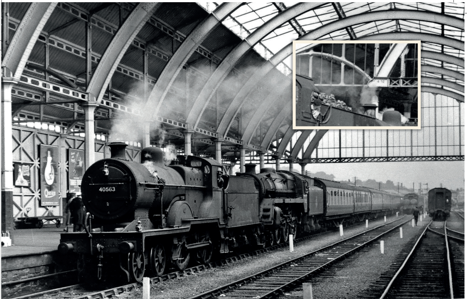
Class '2P' 4-4-0 No. 40563 and BR Class 5 4-6-0 No. 73050, with the Up 'Pines Express' on July 3, 1954, are brought carefully to a stand just short of the buffers. The two rows of white-painted posts at track level are boxed casings protecting water standpipes used for cleaning and servicing coaching stock berthed in the siding adjoining the running line. IVO PETERS, COURTESY JULIAN PETERS. Inset: The 'Paint Date' 4/52 indicated when BR (WR), which had gained commercial control in April 1950, applied the Western Region house colours of brown and cream to the station.
