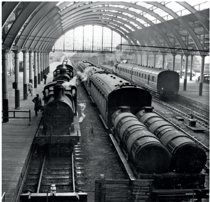
Class '3F' 0-6-0 No. 43441 and '7F' 2-8-0 No. 53806 have arrived with an express from Bournemouth. On the right, 2-6-2T No. 41241 prepares to leave for Bristol Temple Meads. Photographer Ivo Peters took the view from a first-floor window. The gas-cylinder tank wagon was used to refuel the cookers serving the dining cars, and wooden platforms, which covered cellars and stores at basement level. IVO PETERS, COURTESY JULIAN PETERS.
