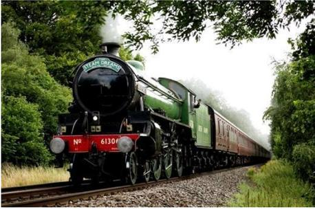
Built for the London & North Eastern Railway, 61306 Mayflower is one of two surviving B1 Class locomotives. The B1's were designed as mixed traffic locomotives capable of hauling express passenger trains as well as freight traffic. As powerful, go anywhere engines, the B1's worked across most of the UK rail network from East Anglia to Scotland.
