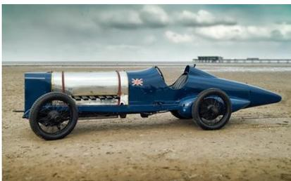
An aero-engined racing car built by the Sunbeam company in 1920, the first of several land speed record-breaking cars with aircraft engines.
