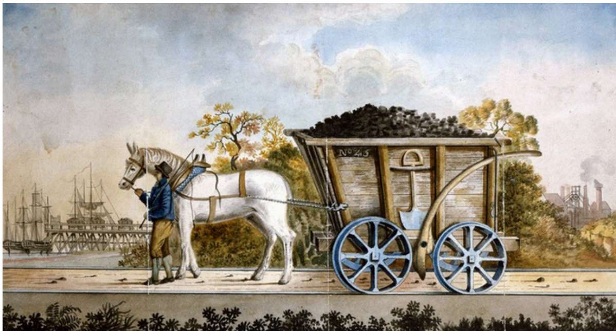
A Waggonway – at Tanfield on Tyneside. The horse provided the means to move the waggon on the level or uphill. Going downhill it was tethered at the rear and the waggonman would control the speed of descent using the large wooden brake lever.
